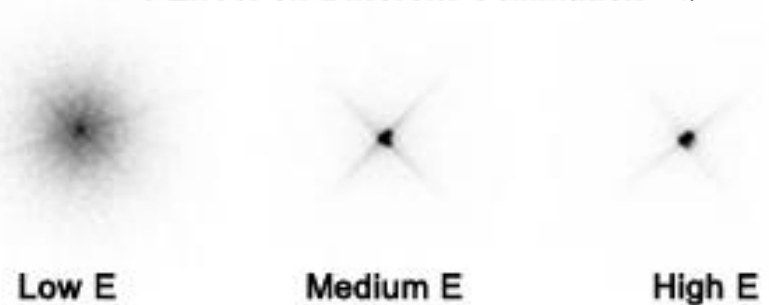
^{131}\text{I} Effect on Different Collimation ( \gamma = 364 keV)
